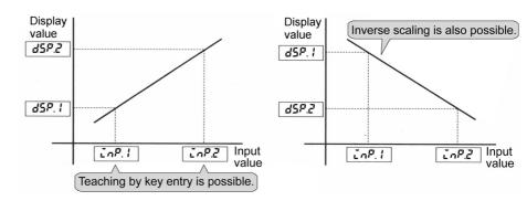
Inverse scaling where readout decreases with increasing input is also possible.
