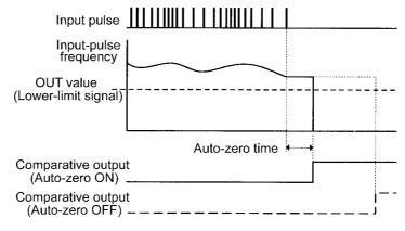
To eliminate such a situation, K3MA-F has an **auto-zero** function that shifts the input pulse frequency to zero forcedly when no pulse is received for a predetermined time.
