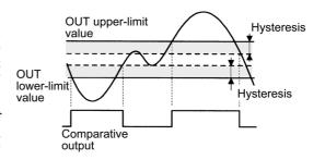
Combinations of comparative output 1 and 2 offer the possibility of producing a wide variety of actions including upper-limit + another upper-limit actions, lower-limit + another lower-limit actions, and two-level outside-the-range actions.
