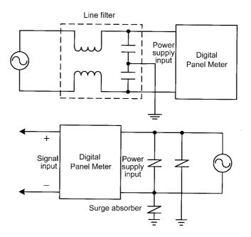
(3) To prevent inductive noise, separate the terminal block wiring for the product from high-voltage or high-current power lines. Do not route the wiring for the product in parallel with or tie it in a bundle with power lines.
