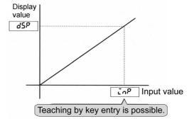
To allow a readout of 10.000 when the input value is 4.2 kHz (= 4200 Hz), for example, set the parameters as follows.
